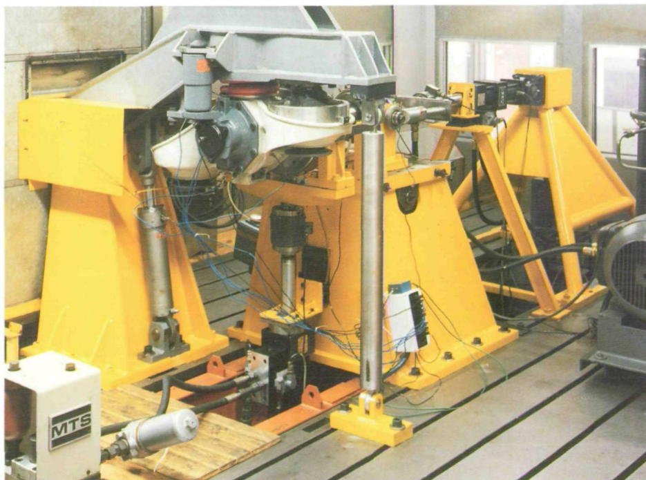
Fig 2 Test rig for high speed train bearings — THISBE
