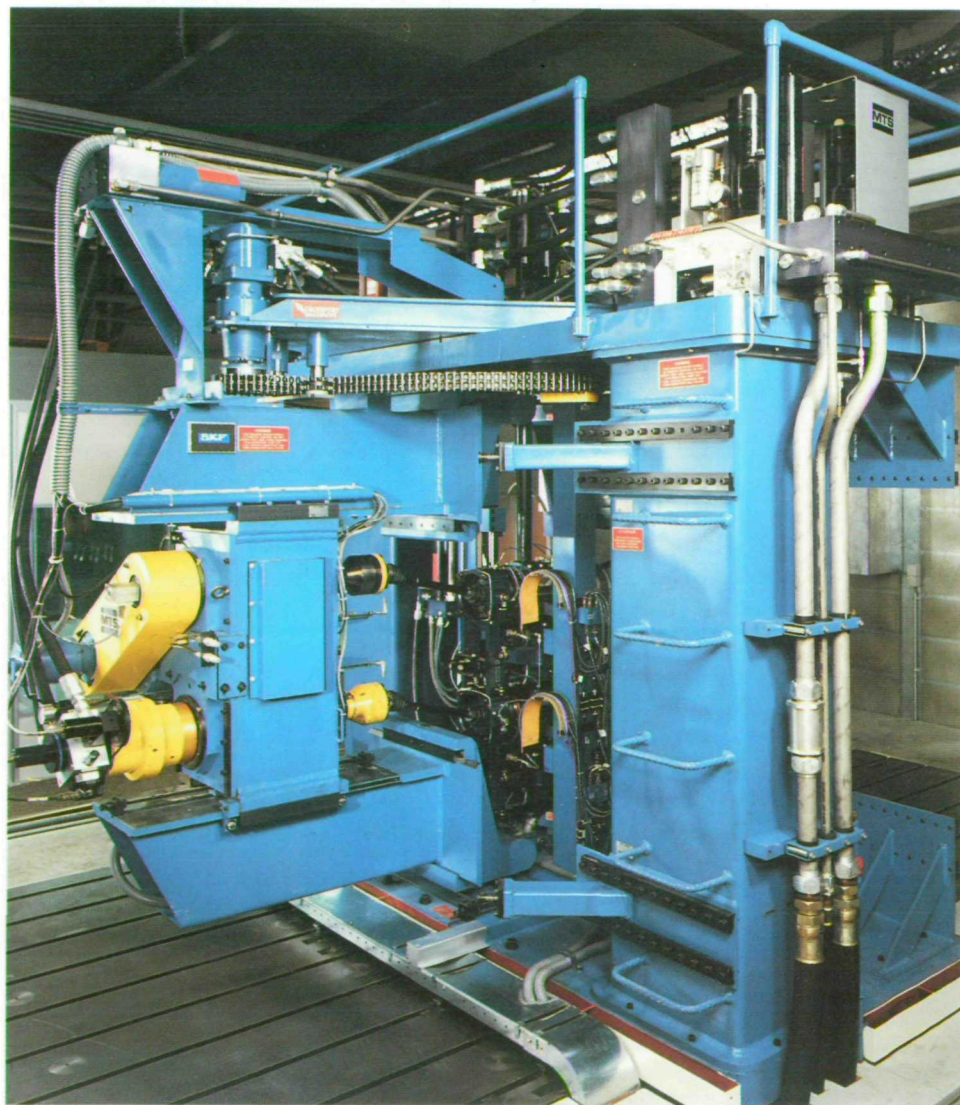
Fig 1 Dynamic testing and analysis system for automotive driven wheel bearing unit arrangements — DYANA
