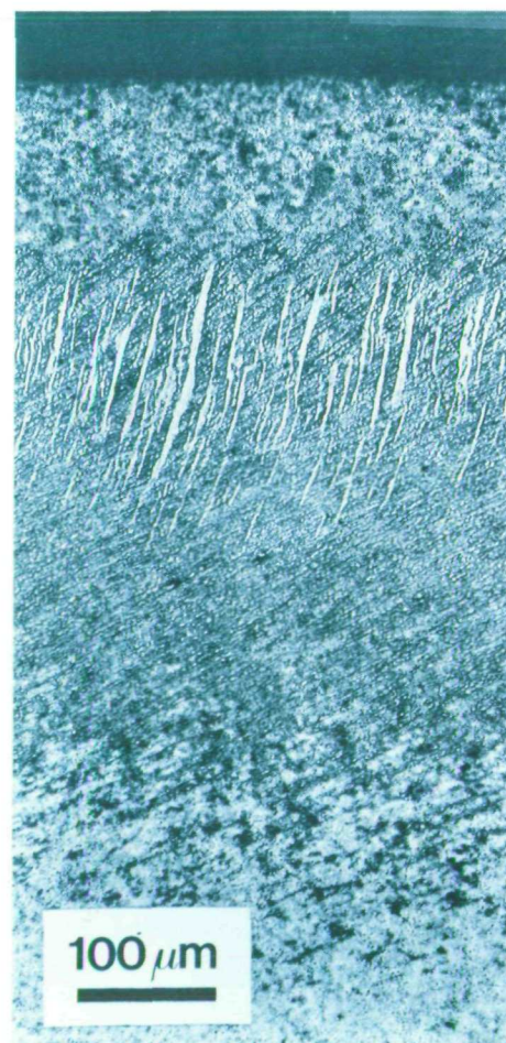
Fig 11 Optical micrograph of axial section through centre of ball raceway of a tested unfailed 6309 inner ring, showing zones of structural changes. Test conditions: maximum contact stress: 3800 MPa, inner ring rotational speed: 6000 r/min, operating temperature: 53 °C, full film oil lubrication. Test time was equivalent to 660 million revolutions
