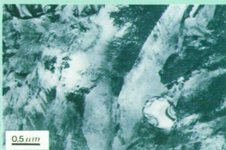
3 Typical mid-ribbed martensite (high carbon, high temperature)
