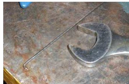
Figure 9: Bent wire with sharp point for feeling surface damages on a bearing.
