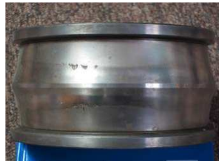
Figure 8: Surface distress and small spalls.
