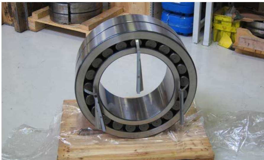
Figure 5: To find the true internal radial clearance, you need more than one set of feeler gauges.
